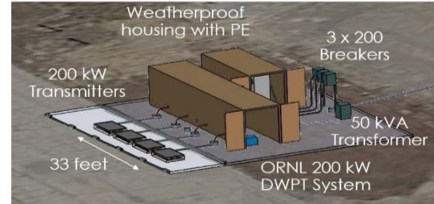
ACM deployment of 200 kW DWPT system with 4 roadway integrated transmitters and roadside equipment
