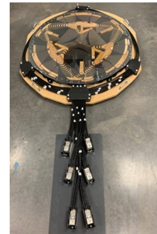
Laboratory development of the 100/300-kW interoperable ground coupler (750 mm diameter)
