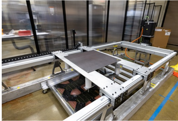
Laboratory development of 200 kW, 20 MPH dynamic wireless charging emulator
